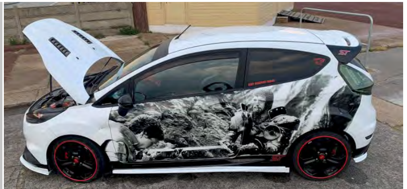
Maxton design abs sprint splitter painted frozen white paired with TRC Ally splitter and fins also painted frozen white, TRC ABS and Alloy side splitters with fins and rear spats also painted frozen white
