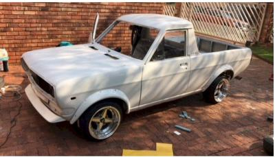
I then replaced all the new Nissan grills for the more nostalgic Datsun grill and round lights, I added a nice chin lip from the Golf MK1. Flushed the rear bin top edging, welded all the holes closed as well as the door handles and petrol cap.
