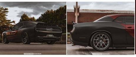
The scat pack comes with a 6.4L v8 engine, I've added a flex-fuel kit to run E85, a full exhaust system from modern muscle extreme, and it's on K-sport Coilover and wrapped by sticky graphics.
